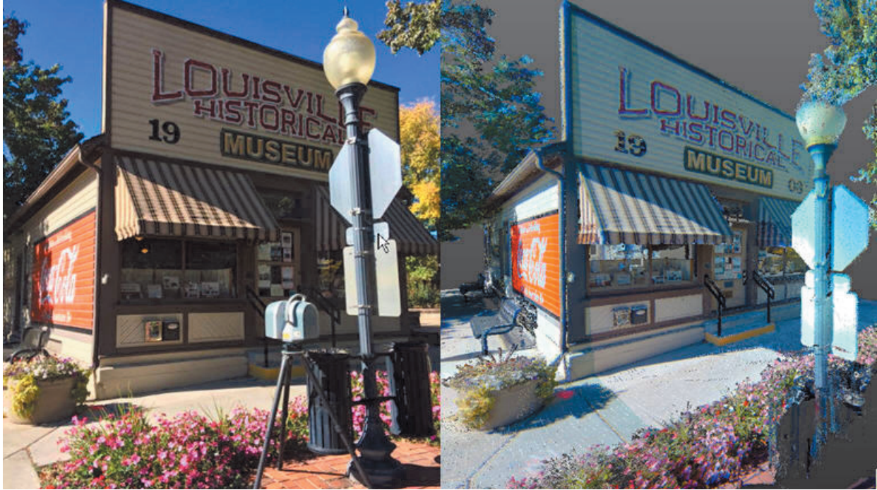
Figure 3: TX6 colored point cloud of building exterior.
