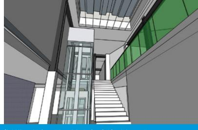
SketchUp model of new stairs and elevator from first floor to basement.
