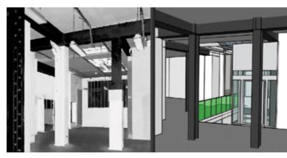
Trimble TX8 scan of original entrance and SketchUp model of new elevator to the basement.
