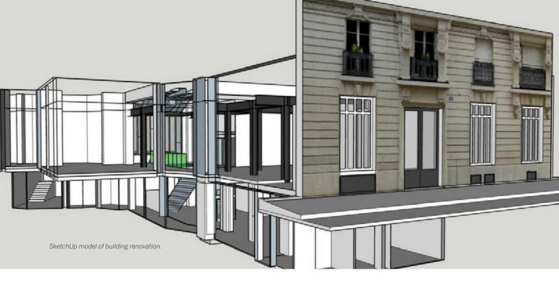
of the façade from a greater distance: 138 million points per scan, with the same 2mm accuracy on all surfaces, even at greater distances.
