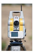
angles to the reflectors located within the telescope's field of view. This function requires neither precise collimation to the reflector nor distance measurement, significantly increasing measurement speed. Ideal for subsidence, displacement or deformation monitoring where vertical or horizontal movements are critical.
